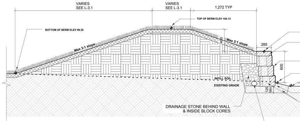
ALLAN BLOCK (AB) WALL SYSTEM SUPPLIER SHALL PROVIDE STAMPED, ENGINEERED SHOP DRAWINGS FOR ALL ALLAN BLOCK (AB) RETAINING WALLS. INSTALL ALLAN BLOCK UNITS PER MANUFACTURER'S SPECIFICATIONS.
